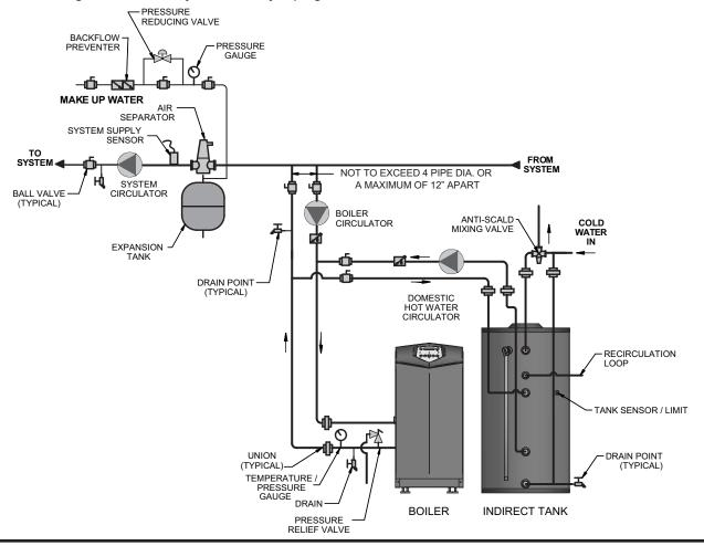
Figure 3-4 Multiple Tank Connections
